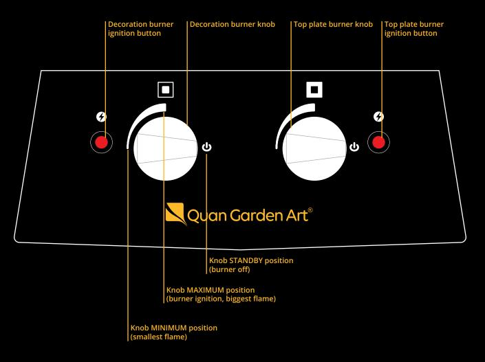
Note! After turning off the burners, wait approximately 10 minutes before reigniting the burners. After turning off the burners, always turn off the main tap on the gas cylinder and the tap on the appliance!
